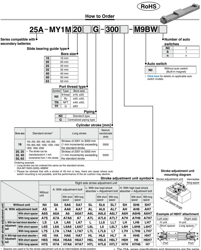
Spacers are used to fix the stroke adjustment unit at an intermediate stroke position
