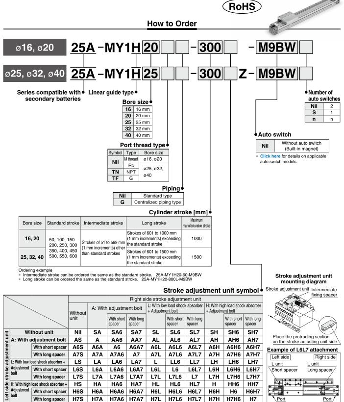
\* Spacers are used to fix the stroke adjustment unit at an intermediate stroke position.
