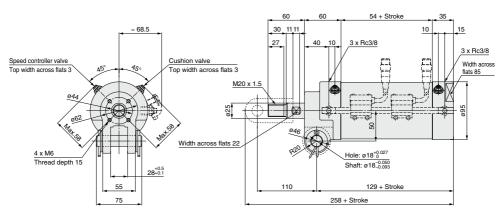
The specifications of the end bracket (double knuckle joint with pins) are the same as those of the standard model.
