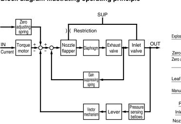
generated by means of the input current at lever fulcrum (2), the output air pressure proportional to the input current will be obtained.
