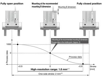
\*1 When mounted on an MHZ2 (ø6) air gripper
