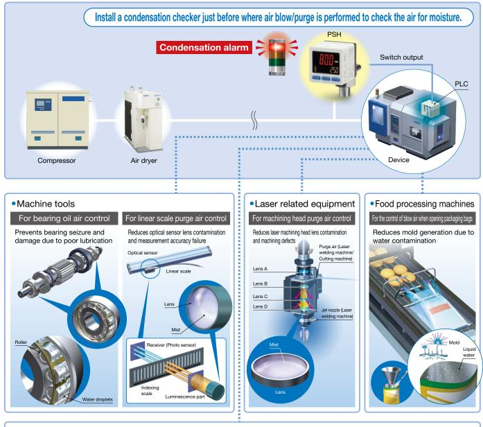
• A solution to condensation, water droplet, and humidification problems in general pneumatic circuits!
