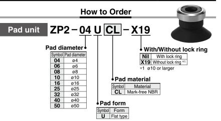
\* The lock ring is shipped together but does not come assembled.
